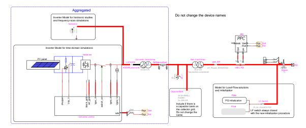
Figure 1 General structure of WECC PV park model
