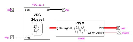
Figure 3 DC-AC converter block inside the inverter hardware model (detailed model version).
