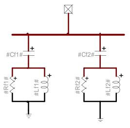
Figure 9 "shunt ac harmonic filter" block.
