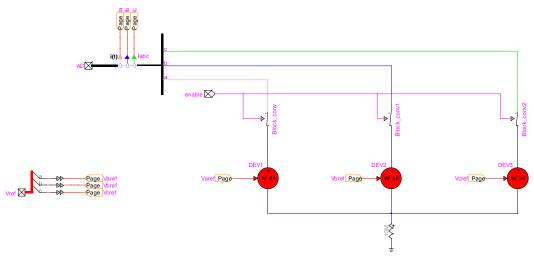
Figure 8 Voltage source model to support REGC\_C model.
