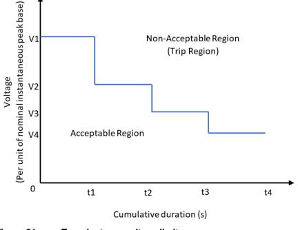
Figure 21 Transient overvoltage limits.
