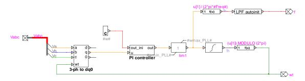
Figure 12 EMTP diagram of SRF PLL.
