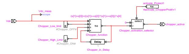
Figure 23 dc overvoltage protection block.
