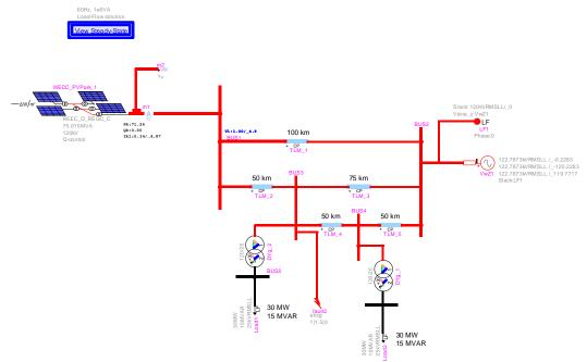
Figure 26 EPRI aggregated PV park network.
