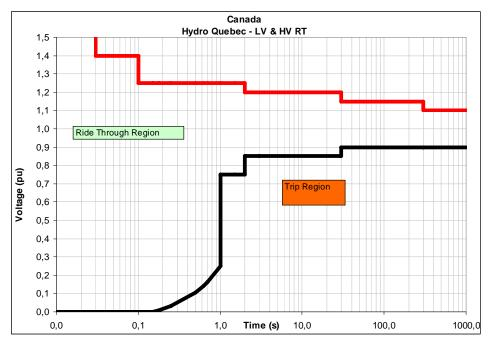
Figure 20 LVRT and HVRT requirements [10].
